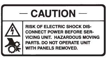
Located on the right, left and rear panels. (part # W0600218)
